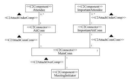
Fig. 13. The C2-style architecture depicted in Figures 7 and 11 expressed in "constrained" UML. Component interfaces have been omitted to draw attention to the stereotypes defining the different architectural elements. For clarity, we show the resulting topology among classes (i.e., component types) rather than their instances.
