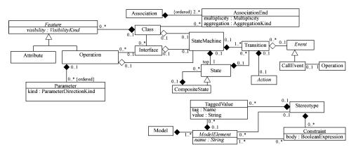
Fig. 4. Simplified UML meta model (adapted from Object Management Group [2000]). Italicized classes are abstract (i.e., noninstantiable) classes. All classes are subclasses of *ModelElement* (except *ModelElement* itself); this relationship is not shown.
