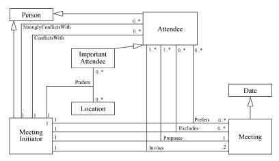
Fig. 8. UML class diagram for the meeting scheduler application. Details (attributes and operations) of each individual class have been elided for clarity.
