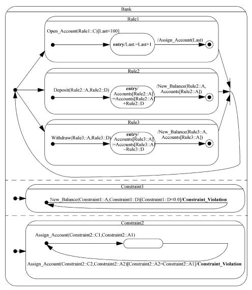
Fig. 18. UML state machine representation of Rapide Bank component.
