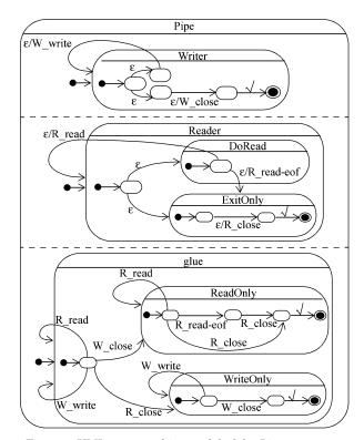
Fig. 16. UML state machine model of the Pipe connector.
