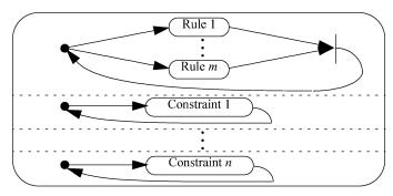
Fig. 17. State machine template for modeling Rapide component behaviors and behavior constraints in UML.
