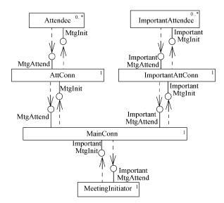
Fig. 11. UML class diagram for the meeting scheduler application designed in the C2 architectural style.
