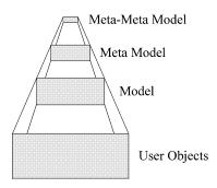
Fig. 2. The four-layer metamodeling architecture of UML. The diagram qualitatively depicts the increase in the sizes of the modeling spaces at each level. For example, the single *meta-meta model* can be used to define a number of *meta models*, such as UML's, which can, in turn, be used to *model* countless *user objects*.
