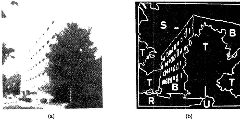
Figure 19. (a) Image of an outdoor scene; (b) Ohta's [1985] resulting labeled image, with S = sky, T = tree, B = building, R = road, U = Unknown. (Used with permission of Pitman Publishing; © Pittman Publishing, 1985.)
