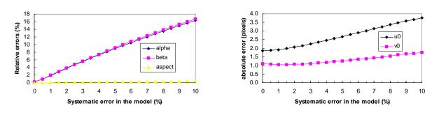
Figure 9: Sensitivity of camera calibration with respect to systematic spherical non-planarity
