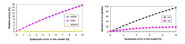
Figure 10: Sensitivity of camera calibration with respect to systematic cylindrical non-planarity
