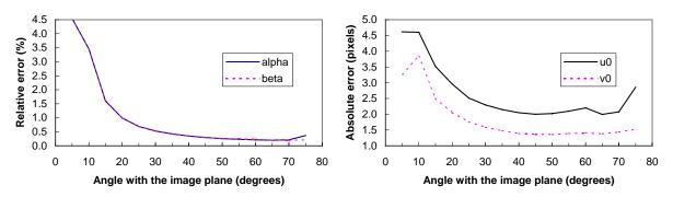
Figure 3: Errors vs. the angle of the model plane w.r.t. the image plane
