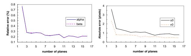
Figure 2: Errors vs. the number of images of the model plane
