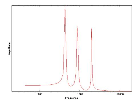
This spectral decomposition correctly shows that the waveform is composed of sine waves at 440, 880, and 2000 Hz.
