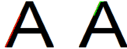
Figure 7: An example of the process of finding the top left corner of "A". The image on the left shows the path from the bottom in red and the image on the right shows the path from the top in green.
