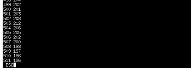
Current sample output of the program: Grayscale pixel values for an individual column of data in a pgm image of an airplane. **Original Image:**
