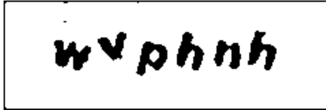
Figure 4: Captcha, after a few rounds of median-filtering. The shape is less sharp, but noise is decreased.
