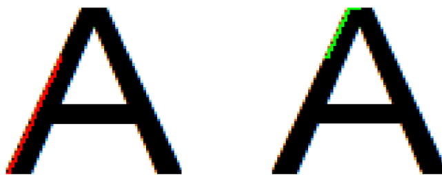
Figure 7: An example of the process of finding the top left corner of "A". The image on the left shows the path from the bottom in red and the image on the right shows the path from the top in green.
