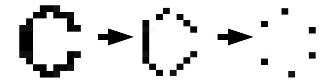
The result is that a letter is simplified into a few line segments connecting key pixels. This procedure is applied to each letter of several different fonts, and information from the results is stored and averaged. Using this, a cache is created to which results from OCR analysis can be dynamically compared.
