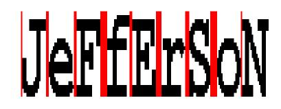
Then, each letter is parsed into portions that pass the vertical line test. After getting rid of unnecessary information, each portion is then transformed into a sum of line segments of different slopes.
