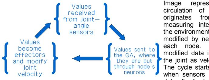
Image representing the circulation of data. Data originates from sensors measuring interaction with the environment, and then is modified by neurons within each node. Finally, the modified data is passed to the joint as velocity values. The cycle starts over again when sensors receive new data after the joints move.
