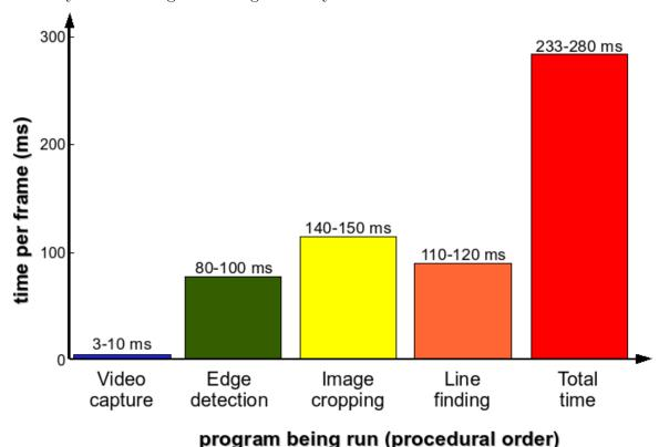
This graph shows that the total processing time per frame is currently around 280ms, a little bit higher than the ceiling of 250ms per frame so that I can interpret sign language in real time at an acceptable pace. However, this calculation does no include line interpretation, so this figure of 280ms is subject to increase.
