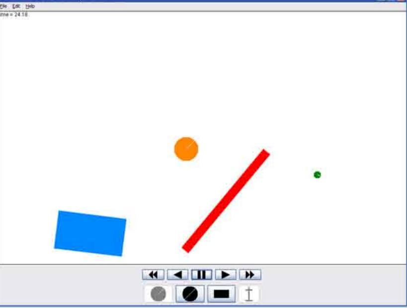
Preliminary Results My program accurately represents projectile motion and collisions with walls without regard to friction, and with an elasticity of one. Once I implement friction and find a good way to determine the elasticity value for each collision, my simulations will seem much more realistic.
