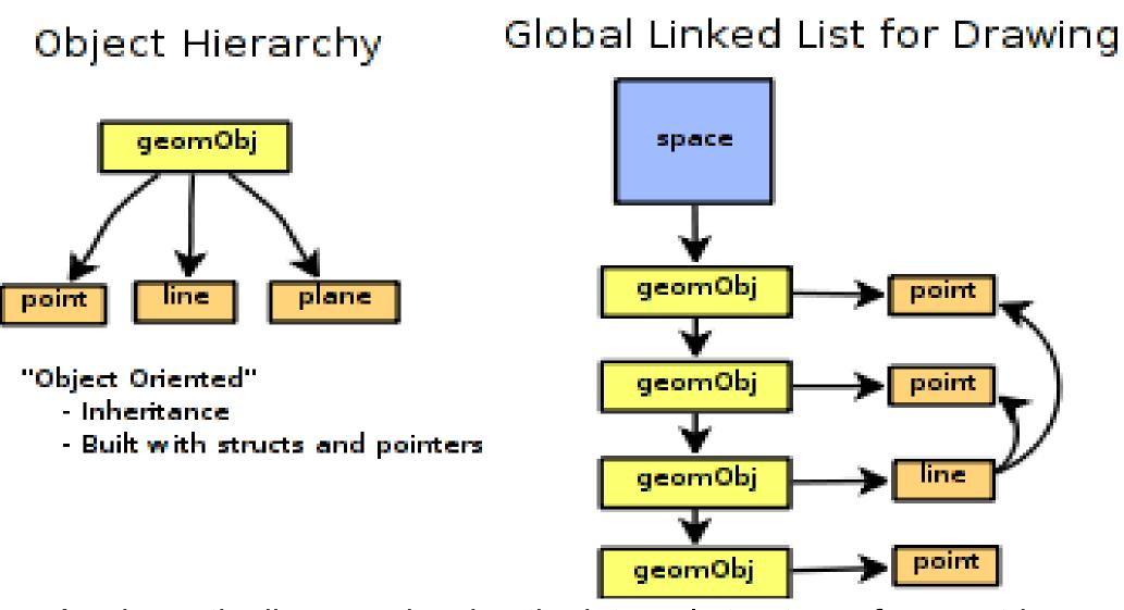
A schematic diagram showing the internal structure of geometric objects, and the structure that stores them for display and calculation purposes.
