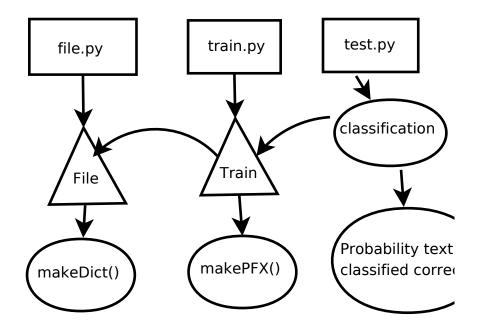
Figure 3: A model of the files and basic operations in the Naive Bayes classifier.
