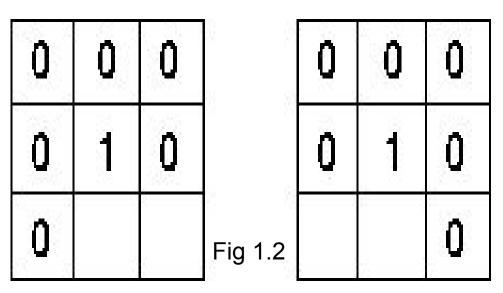
If a 3x3 block matches the matrix, the center pixel is set to 0. By iteratively applying this to a binary matrix until convergence, one can thin an image.
