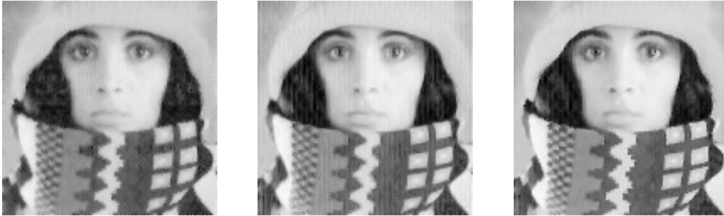
Figure 5. The outputs from the three tested noise reduction algorithms (left to right): Gaussian smoothing, the published edge-sensitive noise reduction algorithm, and my noise reduction algorithm.
