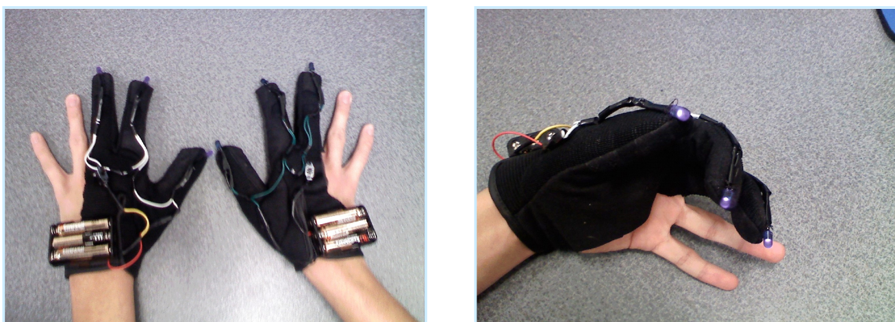
Fig 1. IR LED Glove Final Version
