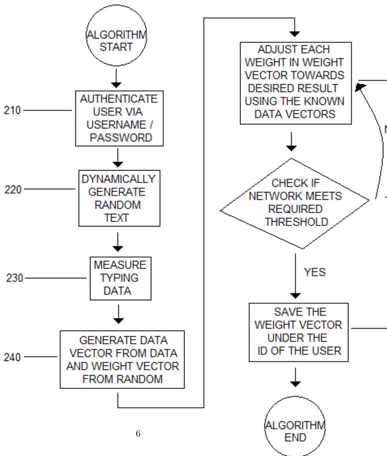
FIG. 3: AUTHENTICATION ALGORITHM FLOWCHART
