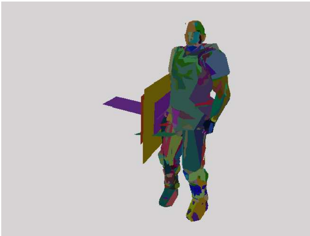
Figure 4: Rendering a skeletal mesh using triangle strips
