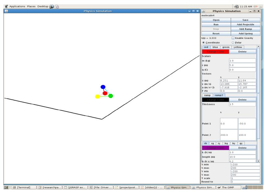
A screenshot of the simulation with a molecule represented by four projectiles connected by springs, and two ramps below. Springs exert forces on attached projectiles, and projectiles can collide with each other and the ramps.
