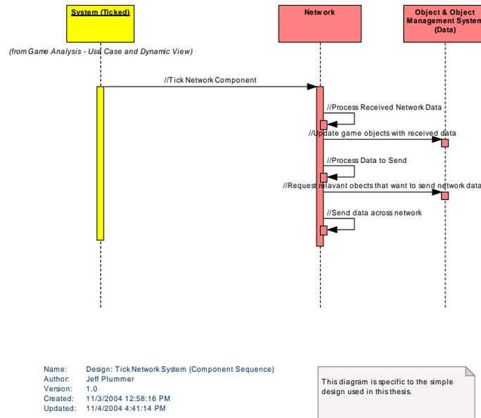
Figure 95 : Design: Tick Network System (Component Sequence)
