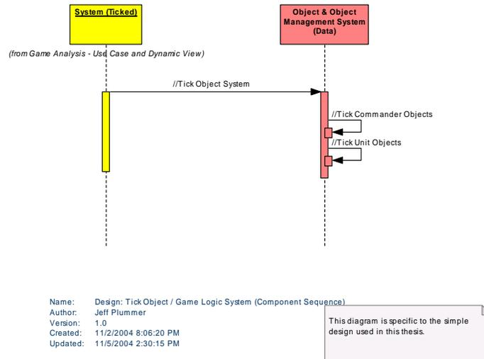
*This diagram shows the sequence of events at the component level that occur to complete the "Tick Object / Game Logic System" use case.*
