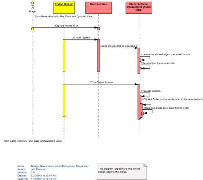
This diagram shows the sequence of events at the component level that occur to complete the "Give unit an order" use case.
