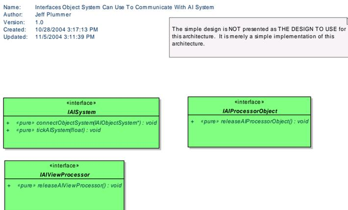
Figure 108 : Interfaces Object System Can Use To Communicate With AI System
