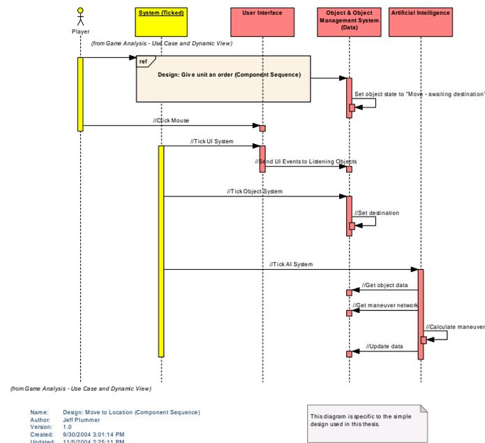
This diagram shows the sequence of events at the component level that occur to complete the "Move to Location" use case.
