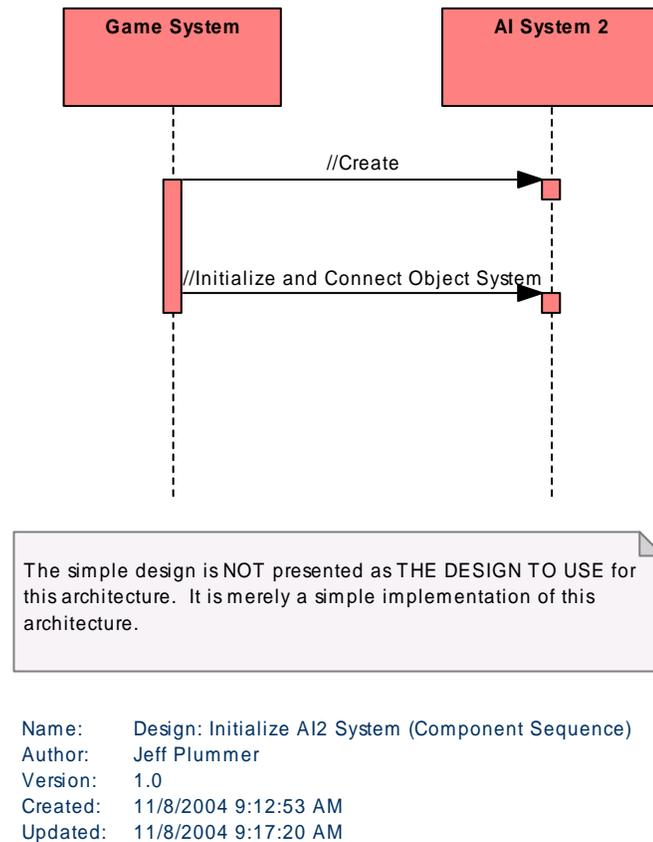
*This diagram shows the sequence of events at the component level required to implement the "Initialize AI2 System" use case.*
