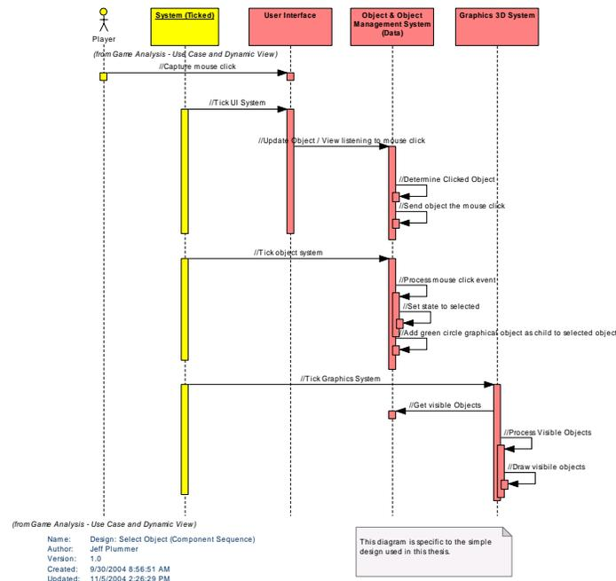
This diagram shows the sequence of events at the component level that occur to complete the "Select Object" use case.
