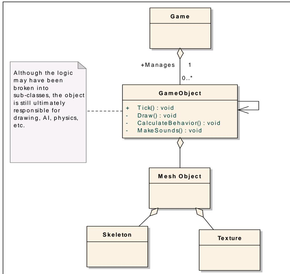
*Figure 4 - Object/Class Level Separation of Logic*
