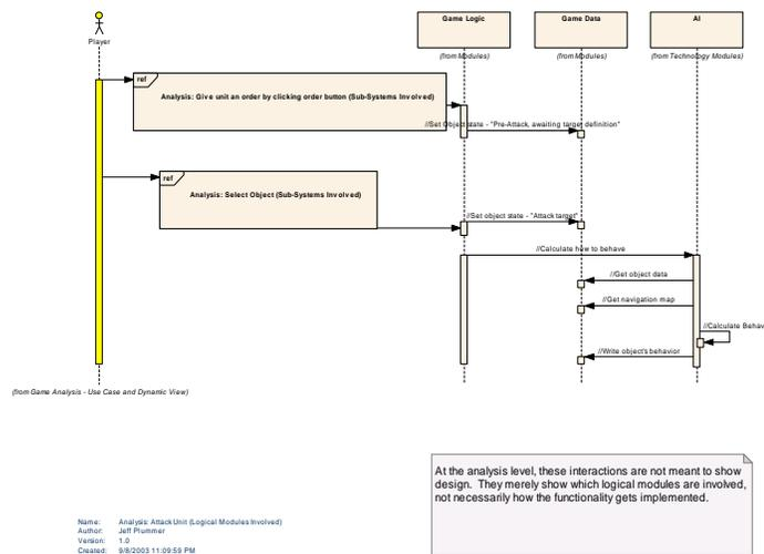
This diagram shows what logical modules are required to perform the "Attack Unit" use-case.
