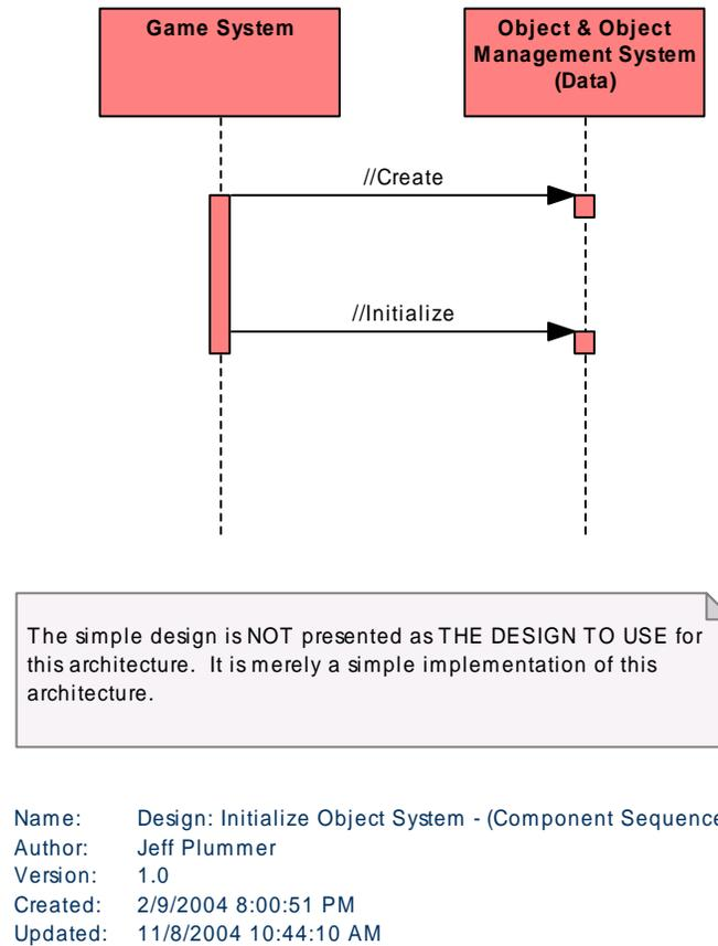
*Figure 147 : Design: Initialize Object System - (Component Sequence)*
