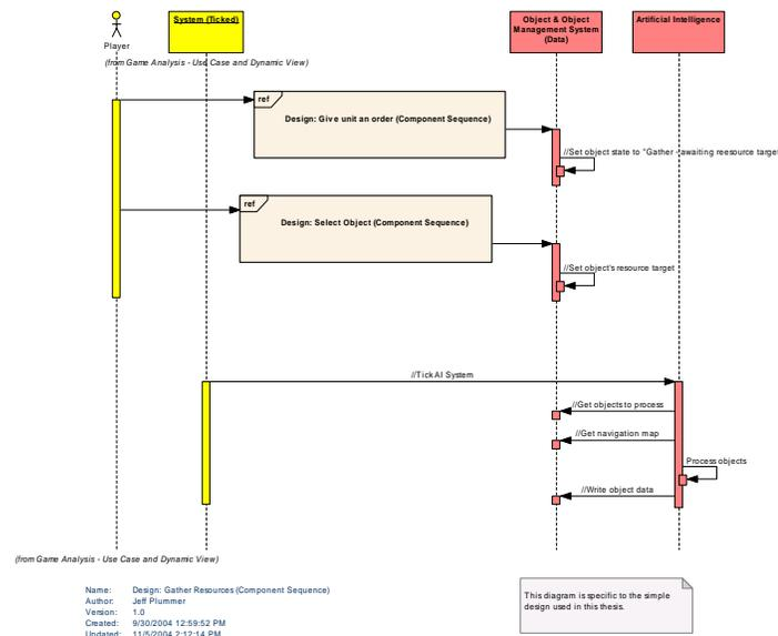
*This diagram shows the sequence of events at the component level that occur to complete the "Gather Resources" use case.*
