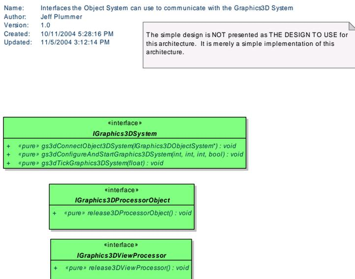
Figure 129 : Interfaces the Object System can use to communicate with the Graphics3D System
