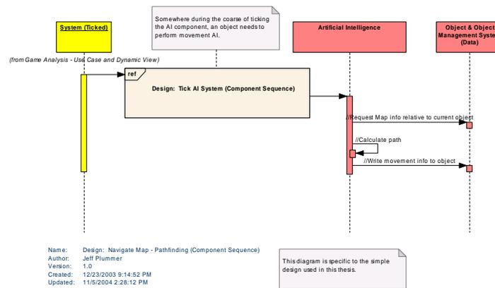
*This diagram shows the sequence of events at the component level that occur to complete the "Navigate Map" use case.*
