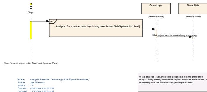
*This diagram shows what logical modules are required to perform the "Research Technology" use-case.*
