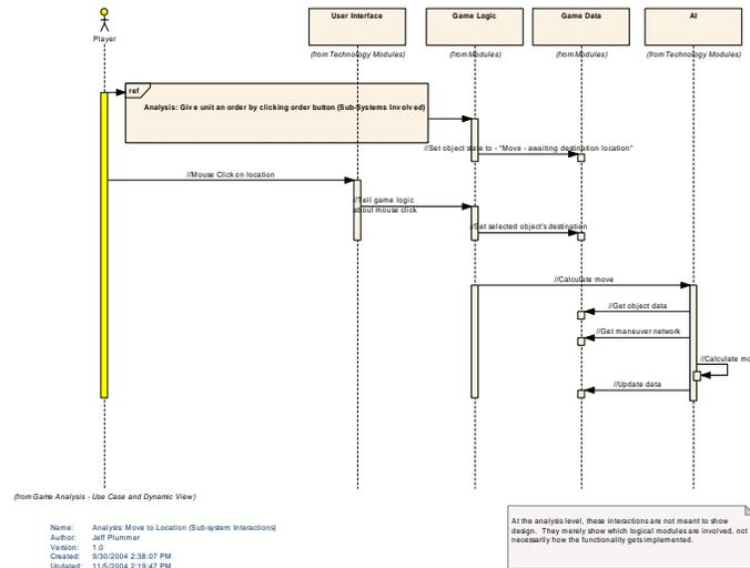
This diagram shows what logical modules are required to perform the "Move to Location" use-case.
