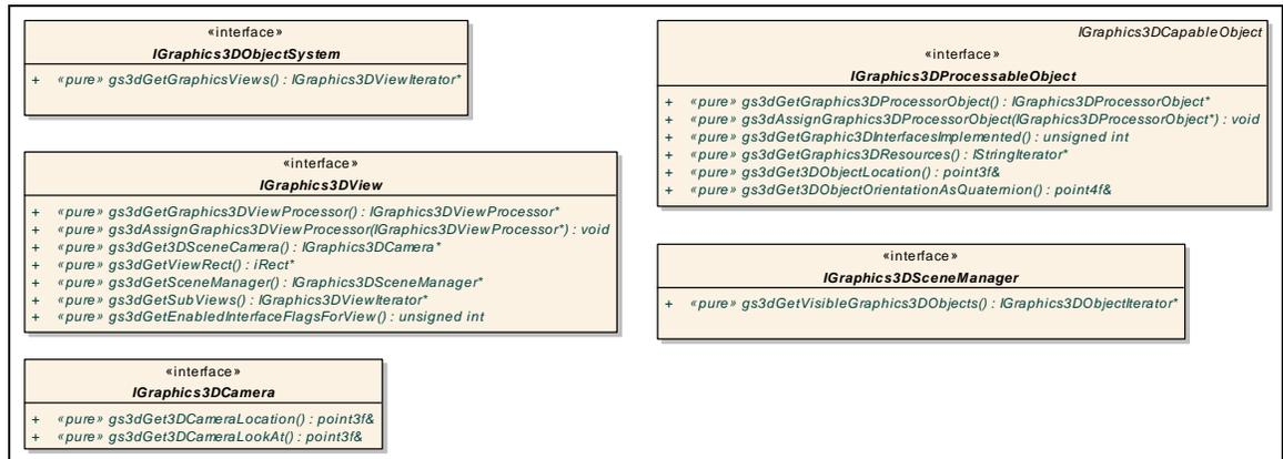
*Figure 41 – Interfaces the Object and Object Management System Must Implement in order for the Graphics 3D Component to Use it.*
