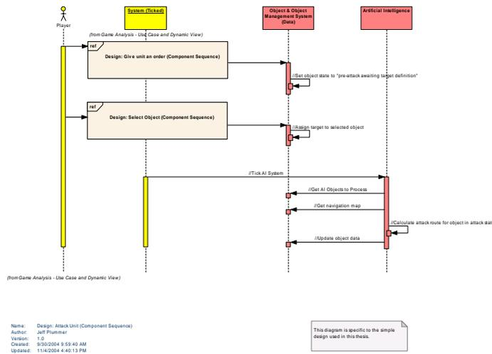
This diagram shows the sequence of events at the component level that occur to complete the "Attack Unit" use case.
