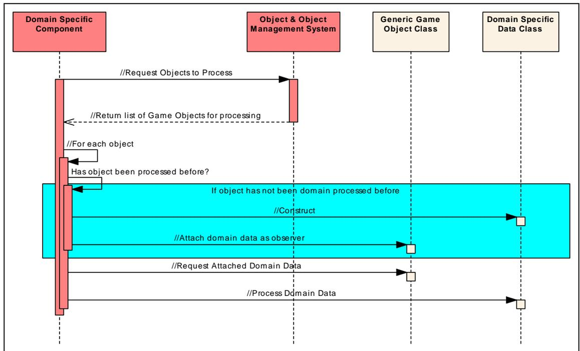
Figure 32-Potential Sequence using a Domain Observer Object
