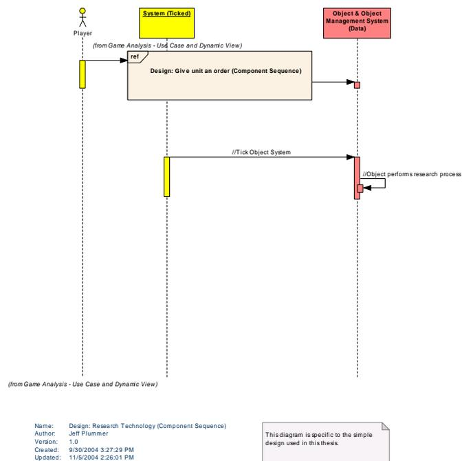
*This diagram shows the sequence of events at the component level that occur to complete the "Research technology" use case.*
