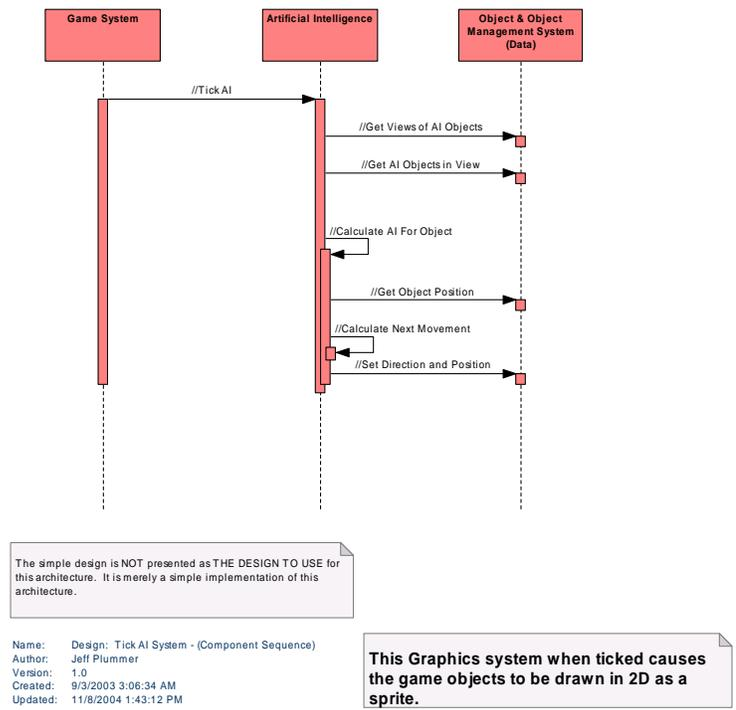
Figure 151 : Design: Tick AI System - (Component Sequence)
