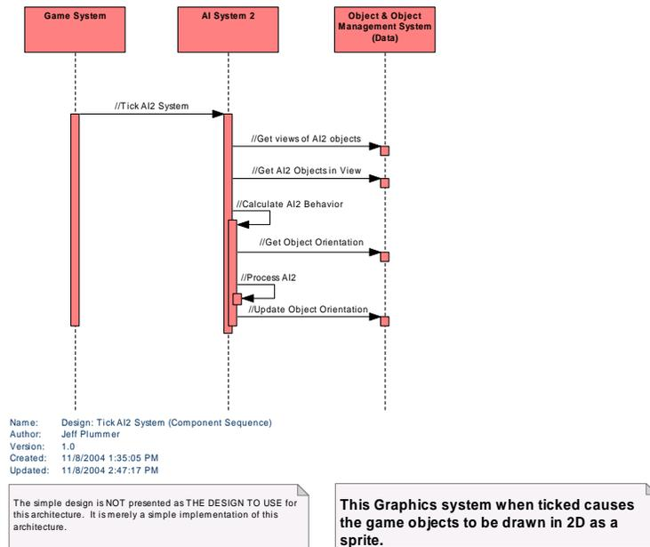
*Figure 153 : Design: Tick AI2 System (Component Sequence)*
