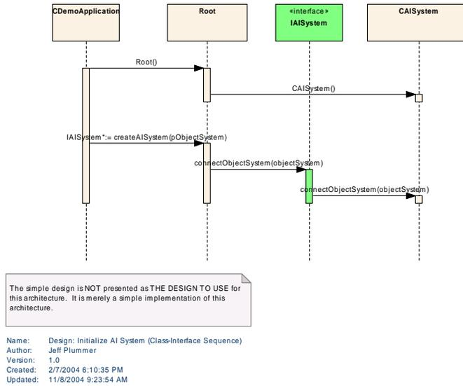
*This diagram shows the sequence of events at the class/interface level required to implement the "Initialize AI System" use case.*
