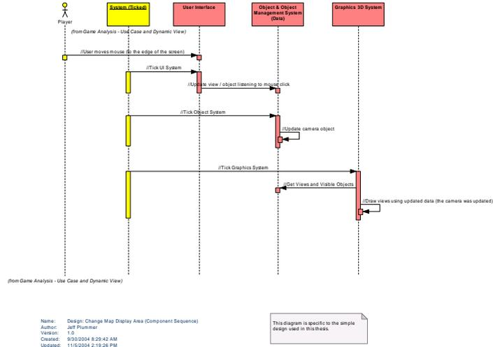
*This diagram shows the sequence of events at the component level that occur to complete the "Change Map Display Area" use case.*
