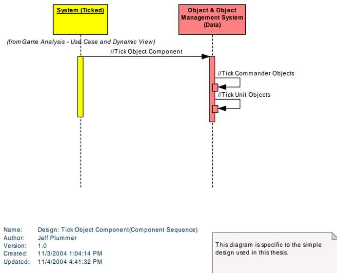
Figure 97 : Design: Tick Object Component(Component Sequence)
