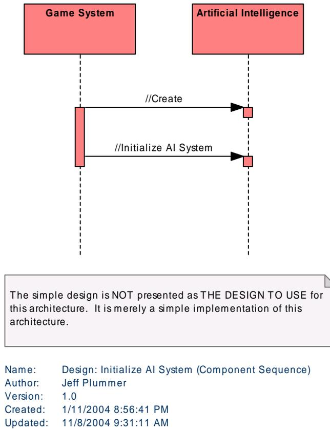
*This diagram shows the sequence of events at the component level required to implement the "Initialize AI System" use case.*
