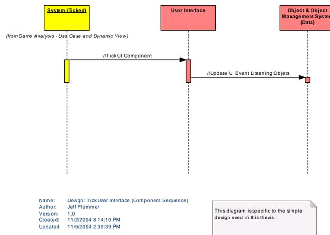
*This diagram shows the sequence of events at the component level that occur to complete the "Tick User Interface System" use case.*
